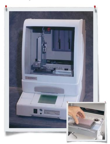
The ProGest Protein Digestion Station is an automated system for in-gel digestion of proteins. All washing steps, enzyme addition and thermal incubation cycles are automatically performed and controlled using a touch screen interface. The unit can also be controlled remotely.
