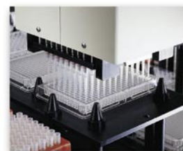
96-channel pipettor accessing a 384-well microplate
