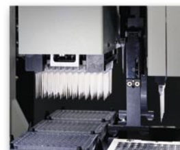
X/Y carriage configured with four independently moving tools
