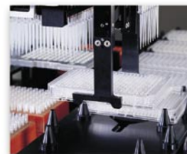
Microplate gripper transporting a 384-well microplate
