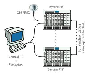
Using Ethernet for communication, physical placement of the GEN DAQ products is flexible and has no additional restrictions. And with the unique fiber optic based Master-Slave module, you can even synchronize mainframes that are hundreds of meters apart, down to the sample level, while the optical synching method used eliminates all ground loop issues.
