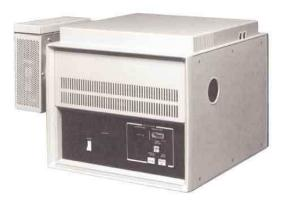
The HP 5970 MSD is a standalone capillary GC detector designed for use with a variety of gas chromatographs. Compact and portable, this requires no cooling water or compressed air, and operates on standard 120v power.
