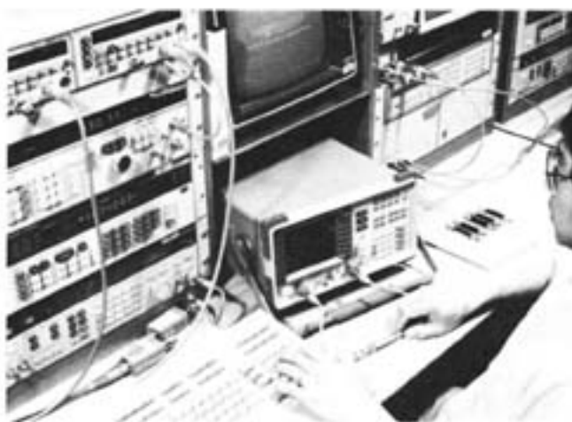
HP 8590 series RF spectrum analyzers have built-in tracking generator option
