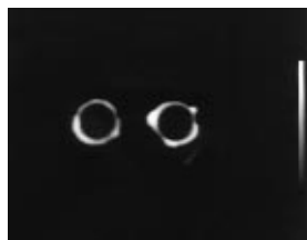
▲ Fluorescent image of oil excited by UV ray.
