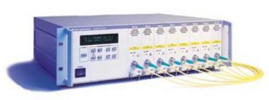
the 315X2 Source Modules supply a minimum of 13 dBm. The modules permit user-selected center wavelengths from 1528 nm to 1610 nm on ITU grid points or the user's custom specification.
