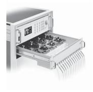
When coupled with the LDC-3916 Multi-Channel Controller, the LDM-4616 provides a configurable, cost-effective solution for multi-channel DWDM signal sources. The tray can also support many popular 980 nm and 1480 nm pump laser diodes for EDFA test applications.
