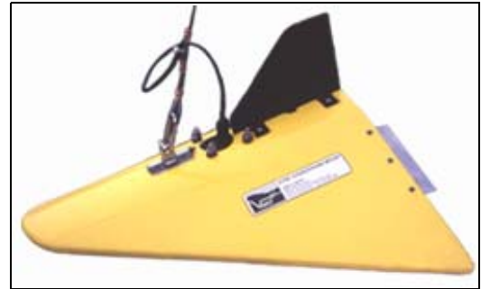
VFIN wing shaped foil
