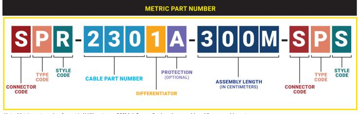
Note: Metric part number format is X.XX meters – 300M defines a 3m length assembly; a 10m assembly part number with the same connectors as shown above is SPR-2301A-1000M-SPS
