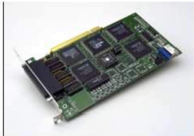
Avtec's MONARCH-E provides 25 Mbps bi-directional performance on a PCI card
