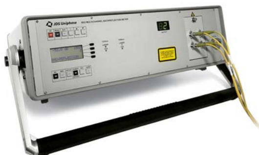
Figure 5: RX3 Series Multimode Multichannel Backreflection Meter
