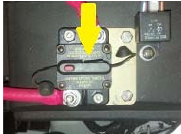
Figure 2: Blade Fuse Holder and Circuit Breaker - Closed Position
