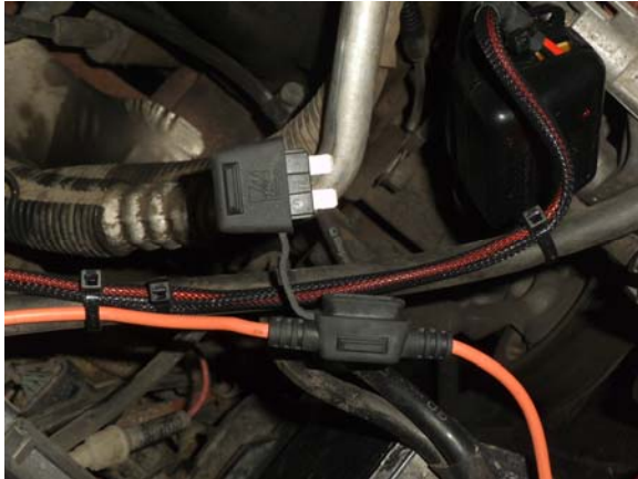
Figure 1: Blade Fuse Holder and Circuit Breaker - Opened Positions
