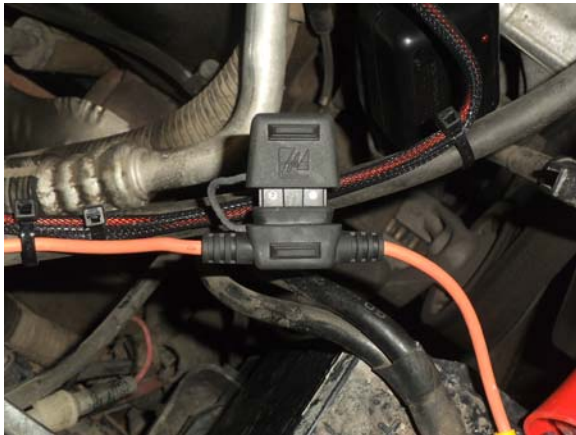
Figure 2: Blade Fuse Holder and Circuit Breaker - Closed Position
