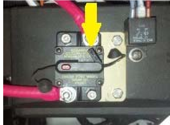
Figure 1: Blade Fuse Holder and Circuit Breaker - Opened Positions
