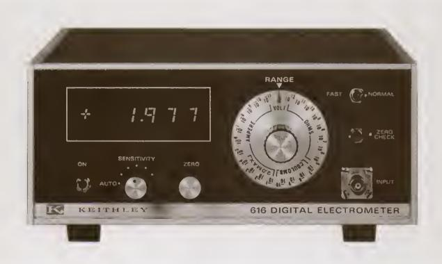
The 616 is an autoranging digital electrometer with sensitivity to  $10\mu V/\text{digit}$  and 0.2% voltage accuracy. The easy-to-read  $3\frac{1}{2}$ -digit LED display includes the convenience of automatic polarity and decimal point. The 616 is essentially a digital multimeter optimized for measurements from high source impedance.
