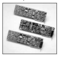
The DAS-16 Series offers 16 single-ended or 8 differential analog inputs with 12-bit resolution. The inputs are switch-selectable for unipolar (e.g., 0 to 10V) or bipolar (e.g., ±10V) input ranges.
