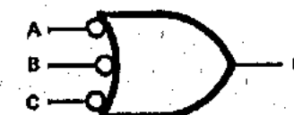
DENOTES "OR" GATE WITH INVERTED INPUTS.
