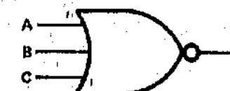
DENOTES "NOR" GATE: "OR" WITH INVERTED OUTPUT.
