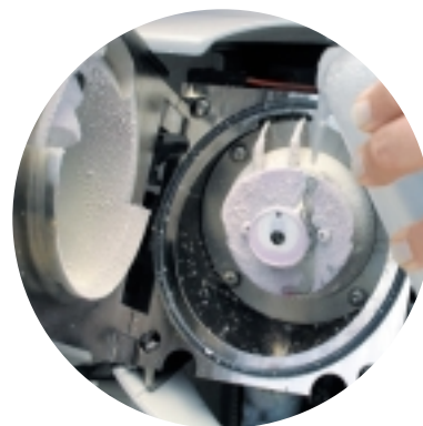
Swing-out spray chamber makes maintenance easier.
