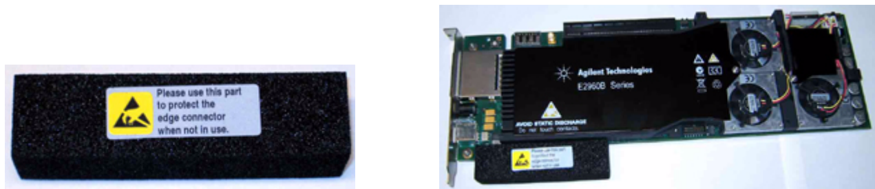
Figure 7 Protective Foam Cover for Edge Connector
