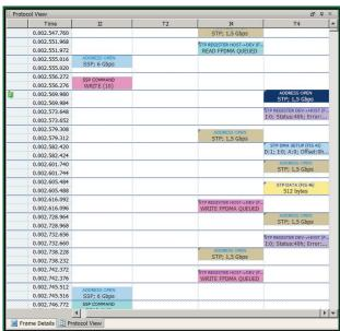
**Protocol View** shows the precise timing relationship of each D-Word in the trace. Useful for tracking the handshaking between products under test.
