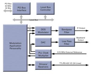
The RTL-VM70 module is part of RT Logic's family of Telemetrix Dynamic Digital Processors. This set of PMC modules support the full spectrum of IF/baseband processing, signal modulation, and digital front-end functions and offer the latest leading edge digital technology.
