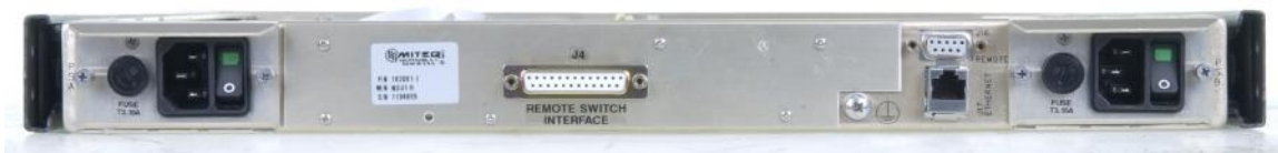
Figure 1-4. Rear Panel, NSU1-R Control Unit
