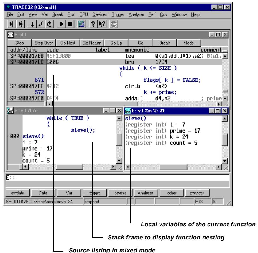
A hierarchical symbol database enables structured symbolic debugging. Symbol names can be up to 255 significant characters long and can be used to show single program
