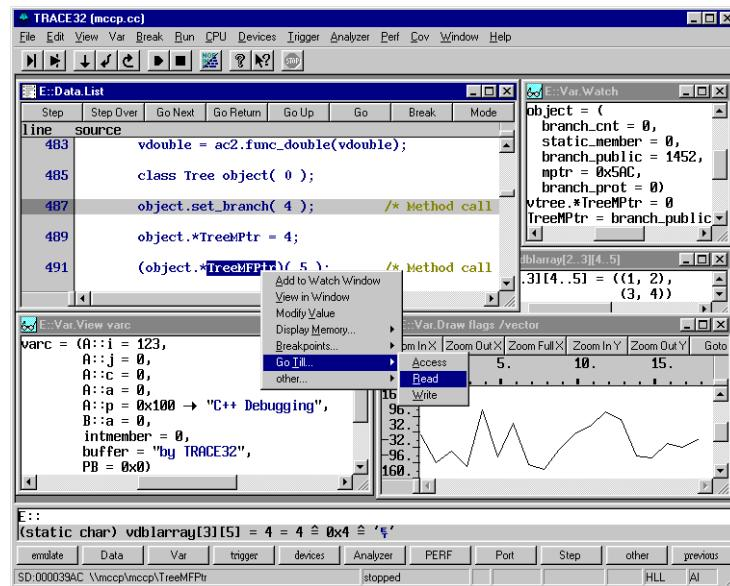
TRACE32 can directly load the output of all standard compilers for C, C++, JAVA, Pascal, Modula2, PEARL and ADA from most compiler vendors. Program display and debugging can be done in assembler, high-level or in a mixture of both. It is possible to con-
