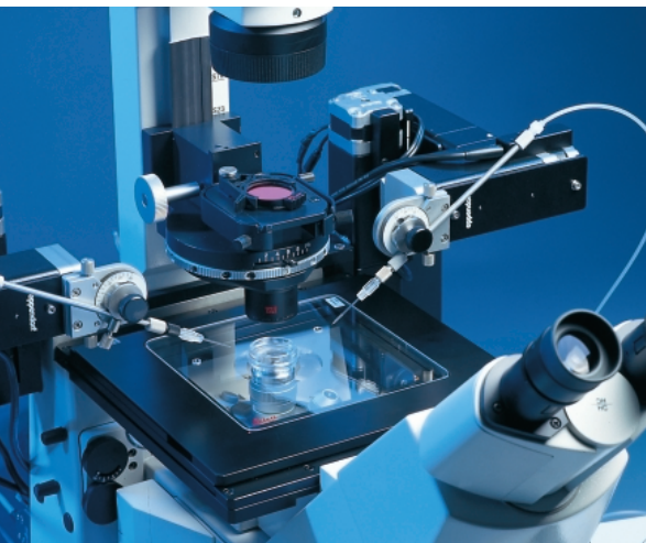
3-plate mechanical stage with glass insert
