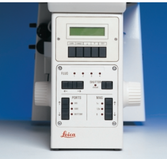
Front control panel for fluorescence filters, shutter, photo TV ports and magnification changer
