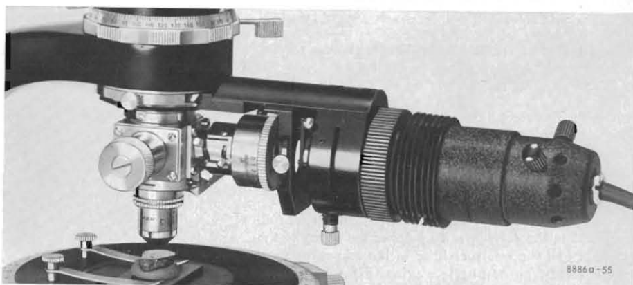
Vertical illuminator with 6 volt 15 watt lamp attachment in position on DIALUX-POL
