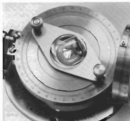
Hollow glass sphere after Waldmann in position on the UT 2 stage. Case with all the accessories at the right
