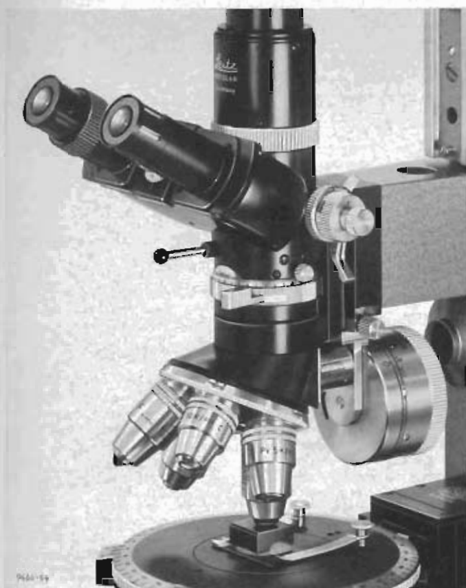
PANPHOT-POL with phase contrast equipment for incident light
