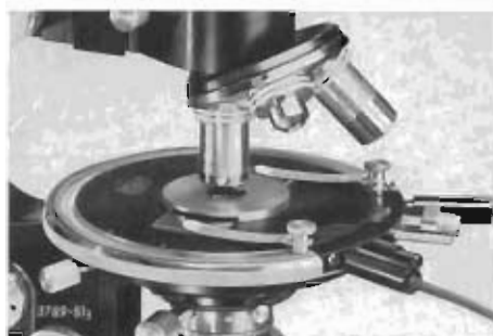
Microscope heating stage with temperature stabilizing chamber in position
