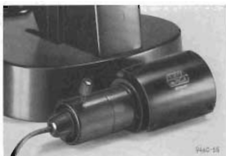
Sodium vapour lamp in position at the rear of the DIALUX-POL base (it is fitted to the LABORLUX-POL in the same way)
