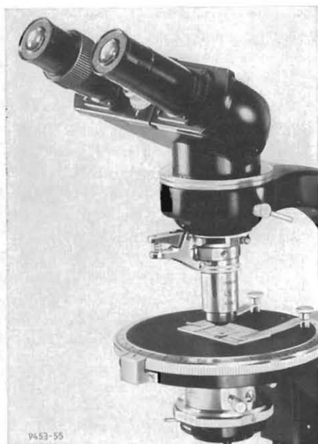
SM-POL with binocular tube 5 20 and objective centring clutch
