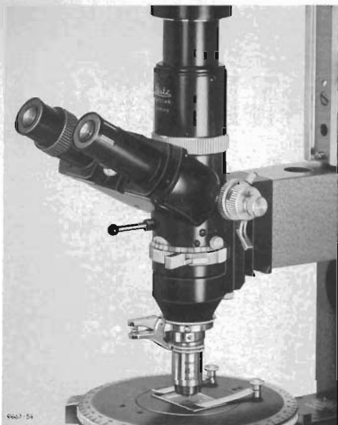
PANPHOT-POL with objective centring clutch
