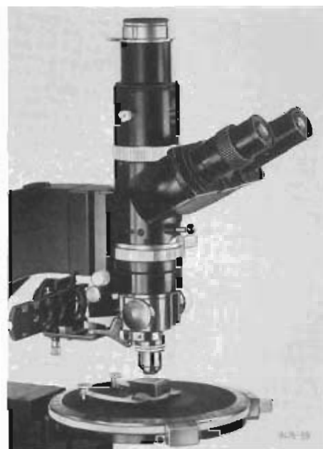
ORTHOLUX-POL with vertical illuminator
