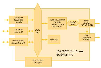
High-Performance DSP Architecture The 104/DSP uses a high-performance 40 MHz DSP to execute real-time motion control algorithms, offloading non-real-time functions to the host. The 104/DSP buffers commands from the host and stores motion and I/O sequences on-board.
