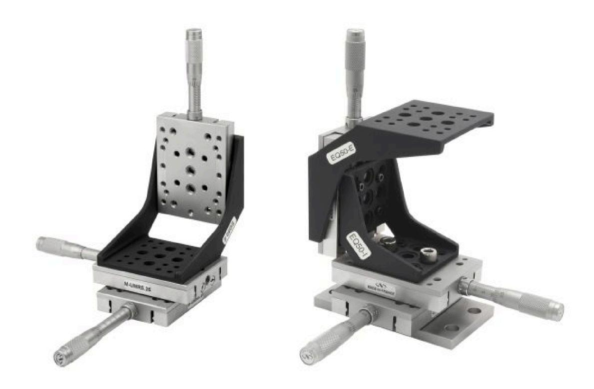
Abundant tapped hole patterns on these stages are included to provide the most options for mounting components on the stage mounting surface. Two stages can be easily stacked to provide XY translation (except the UMR5.5). Z configuration can be assembled using the EQ Series Angle Brackets. Two XYZ configurations of (3) UMR5.25 linear stages with EQ50 angle brackets are shown.
