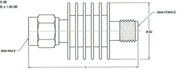
NOTE: To specify Part Number, insert nominal attenuation value in place of dB, i.e., 602-10-1 for 10 dB.
