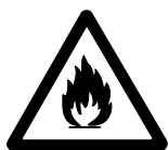
Risk of fire
