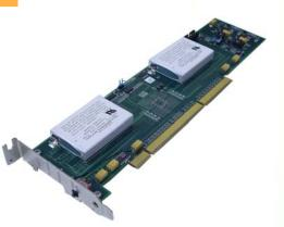
The MM-5428CN is a low profile PCI card with a 64-bit/66MHz PCI interface and 256MB to 2GB of NVRAM.
