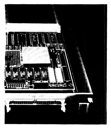
ROM devices, 16 bi-directional parallel I/C lines, three off-board-accessible programmable 16-bit counter/timers, hexadecimal LED status display, and seven interrupt levels with bus arbitration. Designed to serve as a system controller (slot 1). **MVME101**
