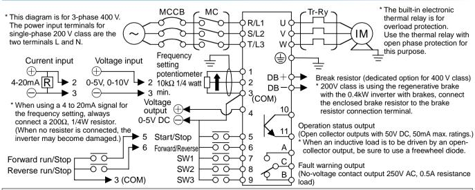
When shipped it is set for control using the operation panel. Parameter settings will have to be changed depending on the control signals that will be used.
