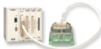
Figure 1. TBX Terminal Block Cabled to SCXI Module
