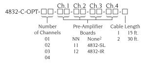
2) The NN code cannot be entered in the Ch. 1 option field, since the 4832-C is sold with at least one pre-amplifier channel in the break-out box.
