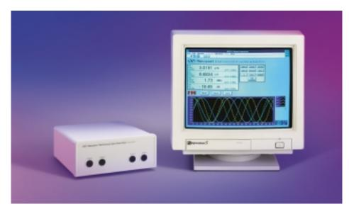
The 4832-C Multi-Channel Optical Power Meter features multi-channel, high-speed and high-precision, NIST calibrated optical power measurements. The system consists of a breakoutbox connected to a PC plug-in board. The breakout box can be located up to 30 feet away from the PC, allowing its easy integration in manufacturing and assembly environments.
