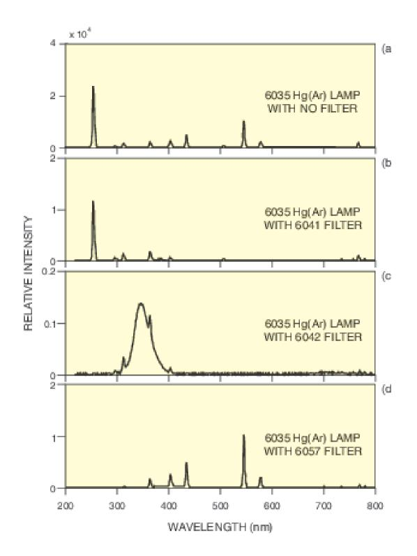
When only certain portions of the lamp's output are required, three different filters are offered to block out the undesired spectral lines. Like the aperture shields, these filters simply slide over the lamp.
