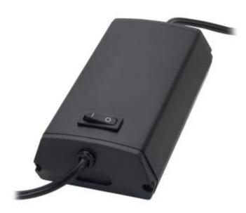
The 6045 AC Lamp Power Supply is designed to operate Neon, Argon, or Krypton pencil style calibration lamps. This power supply is required for lamp operation. This supply regulates variations in output intensity, which has the added benfit of prolonging lamp life. It is rated for 10 mA of output current and has a 110 VAC, 60 Hz input power requirement.
