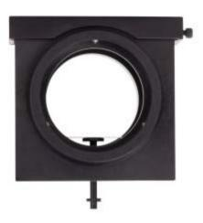
The 71260 Quick Change Filter Holder provide the ability to quickly insert and remove filters in the middle of an optical train. A plunger on the bottom of the holder pops the filter up for easy removal. A light tight cover prevents leakage of ambient light into the enclosed optical path. It holds 1.75 to 2 inch (43 to 51 mm) circular or square filters and has a 1.6 inch clear aperture. 1.5 Inch Series flanges. **^** SHOW LESS
