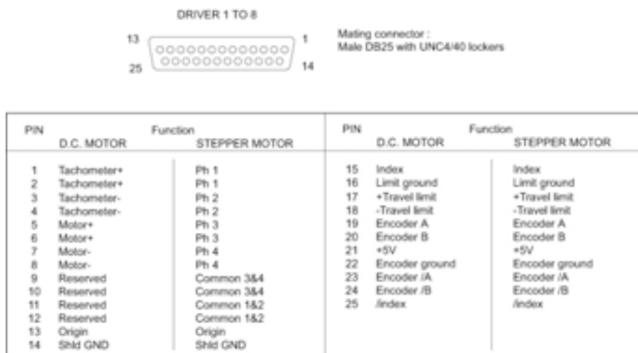
Figure 71:XPS-DRV01 Motor Driver Connectors.
