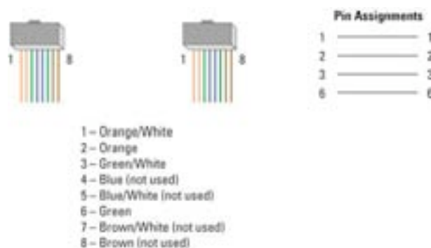
Figure 12: Straight through cables.
