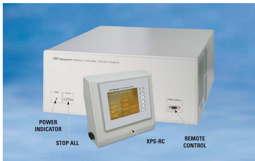
Figure 7: Front Panel of XPS Controller/Driver.
