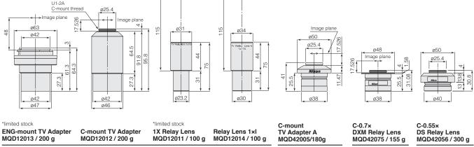
ENG-mount TV Adapter and C-Mount TV Adapter are used in conjunction with 1x Relay Lens.
