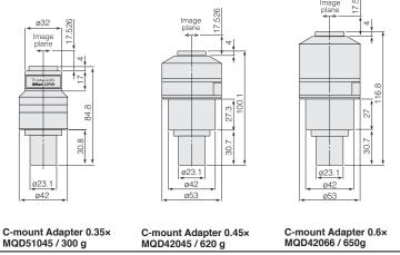
C-mount adapters feature a built-in reduction relay lens, enabling areas equivalent to those seen through the eyepiece to be viewed on the monitor. Adapters for 1/3-inch (0.35×), 1/2-inch (0.45×), and 2/3-inch (0.6×) CCD cameras are available.
