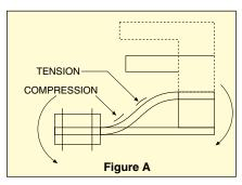
Two typical mounting arrangements are shown below. For high-accuracy applications, reinforcement plates should be slightly harder than the beam material, and the interfacing corners should be sharp. Because of low loads and sensor construction associated with the LCL113G through LCL-816G, in-line loading (Type 2) is not recommended.
