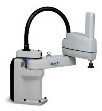
The Adept Cobra™ s800 robot is a high-performance SCARA robot system for mechanical assembly, material handling, packaging, machine tending, screw driving, and other a fast and precise automation. Adept Cobra s-Adept SmartController™ motion controller, w capabilities unmatched in the industry.
