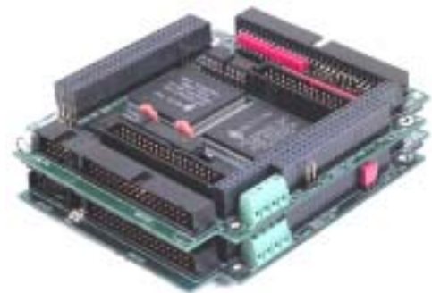
PMAC2A-PC/104 Base Board shown stack with the ACC-1P
