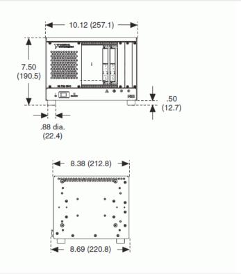
PXI-1031/PXI-1031DC Dimensions (Bottom) in Inches (mm)
