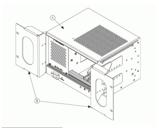
1 PXI-1031/PXI-1031DC Chassis 2 Rack Mount Kit
