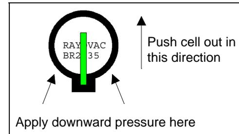
**Figure 14. Battery Removal.**
