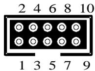
A second serial port, addressable as PC serial port COM2, exists in the form of a 10-pin header on the printed-circuit board near the bottom of the front panel. Pin 1 is the pin closest to the front panel and the bottom of the EPC-7 printed circuit board. The header is defined in the table below.
