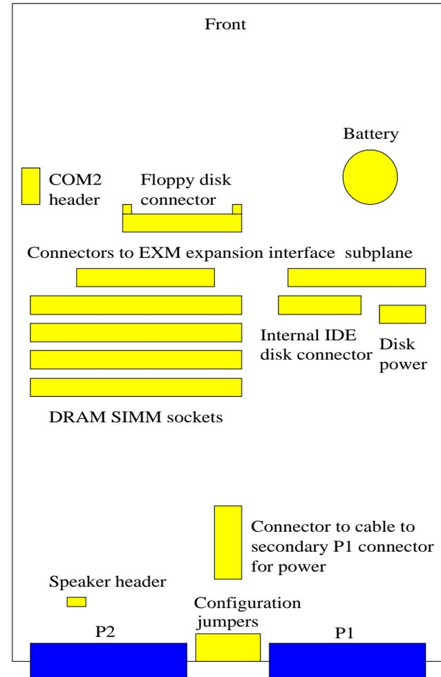
Figure 15. PCB Layout.
