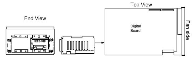
Step **(6)** Plug option cable into option card.
