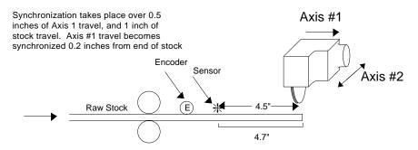
Below, the master cycle length will be set equal to the desired cut length (36" in the example below), which the operator can change by modifying variable Q1. The cut cycle will be a continuous loop, but the first cut will be made 0.2" from the end of the stock to ensure an even first edge. Axis #1 will accelerate to the desired tracking ratio over 1 inch of master travel for all cuts. Assume that the home position of both axes is at position 0".
