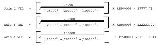
Axes 1, 3, and 4 will start moving at the same time, reach their peak velocity at the same time, start decelerating at the same time, and stop at the same time. Axis 2 will not participate in the linear interpolated move, it does a preset move of 50,000.
