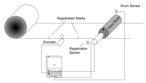
Drum is in the center of 1:1 constant ratio print portion when drum sensor occurs
