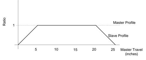
If the master distance specified is too large for the slave distance and FOL RATIO commanded, the slave will never actually reach the commanded FOL RATIO, and the move profile will look similar to that below. Here, the FOL MDIST is 25 inches and the slave is commanded to move 10 inches:
