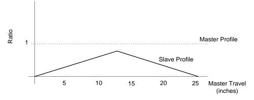
If the master distance is too small for the slave distance and FOL RATIO commanded, the 4000 will not perform the move at all. For example if the FOL MDIST is 25, the FOL RATIO is 1:1, and the slave is commanded to move 30 inches, the move will not even be attempted.
