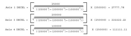
Axes 1, 3, and 4 will start moving, reach their peak velocity, start decelerating, and stop at the same time. Axis #2 will not participate in the linear interpolated move, it does a preset move of 50,000.
