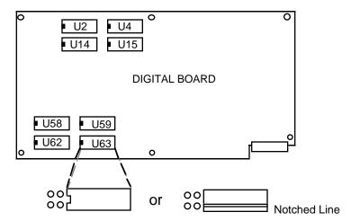
Both RAM and PROM IC's should be installed so that the empty slots are positioned as above.
