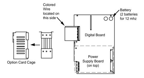
Step ⑤ Slide option card cage into position and plug option cable into option card J1. Attach option card cage to end plate using HEX nuts supplied.
