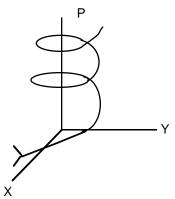
A sewing machine application may require all four axes (X,Y,C, and P). The X and Y axes would direct the sewing head along the required path. The C axis would keep the sewing head pointed into the direction of travel. The P axis would control the speed of the needle, so that an even stitch is made, regardless of path speed.
