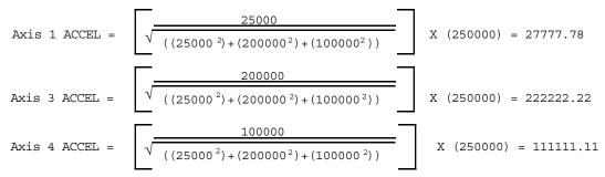
Axes #1, #3, and #4 will start moving, reach their peak velocity, start decelerating, and stop at the same time. Axis #2 will not participate in the linear interpolated move, it does a preset move of 50,000 steps.
