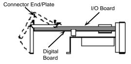
Step ④ Remove the J5 (phone cord) connector (on Digital Board), plug option cable into connector J4 (50 Pin Connector).
