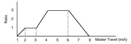
In the example above, FOL MDIST was executed *after* an ACCEL statement. If the ACCEL statement had been the most recent, its slave would use that acceleration to ramp to the new ratio, but the corresponding master travel would be unknown. This may be preferred in velocity based applications such as mixing or pumping, in order to match the acceleration to the motor's torque and load.
