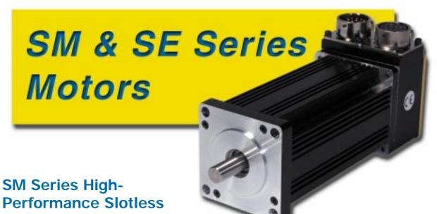
The SM Series brushless servo motors feature a slotless stator design. This design eliminates all detent torque in the motor, allowing the SM Series motors to provide extremely smooth motion, especially at low speeds. The slotless design also creates a higher rotor inertia, which is ideal for applications involving high inertial loads (such as lead screws and belt drives).
