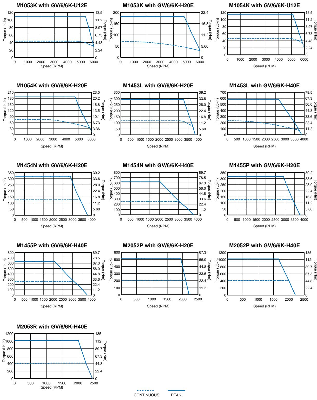
\*Encoder feedback performance shown. Resolver-based systems provide up to an 8% increase of continuous and peak torque at all speeds over encoder-based systems. Refer to the Servo Motors section for more information on resolver motors.
