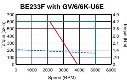
CONTINUOUS PEAK 120 VAC 120 VAC MECHANICAL LIMIT
