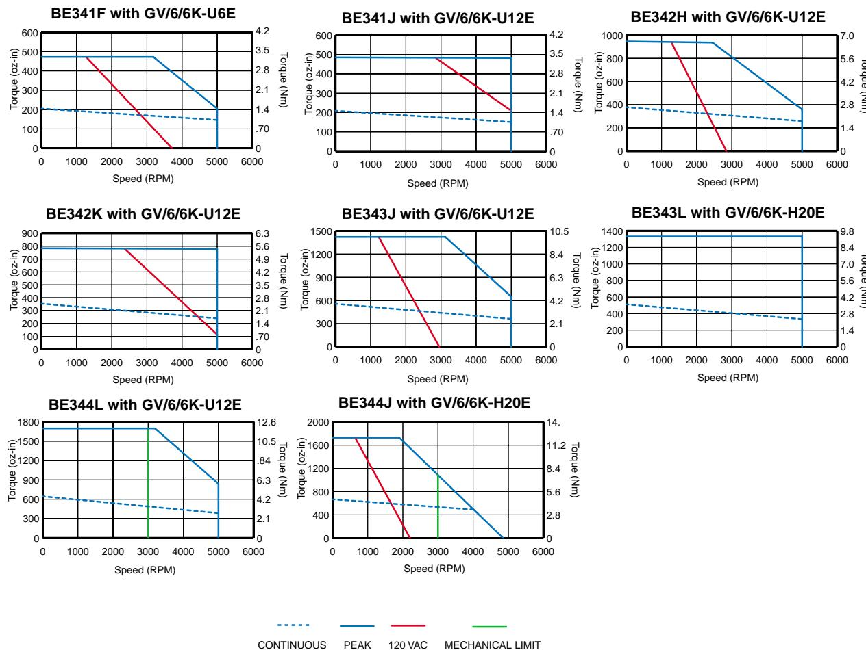
\*Encoder feedback performance shown. Resolver-based systems provide up to an 8% increase of continuous and peak torque at all speeds over encoder-based systems. Refer to the Servo Motors section for more information on resolver motors.
