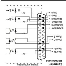
circuit in motor or motor cable MOTOR FAULT Red when drive detects short OVER TEMP Red indicates over temp fault Flashes Red/Green in auto test STEP Green when drive receives step
