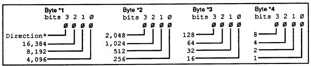
In Q2 mode, this byte indicates the number of steps the motor will move per time interval. In Q3 mode, this byte indicates the velocity that the motor will move per time interval. You can set the time interval with the TD command. In the Q3 mode, the velocity desired per update interval is related to the four hex digits as follows (disregarding the most significant bit which is the direction bit):
