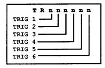
When TR command is used in a buffer, the indexer will get to this command and wait until the input pattern is matched before going on to the next command.
