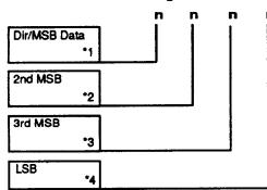
MSB = most significant bit LSB = least significant bit If you want to define data for one axis in a timed data streaming mode, use the configuration spanner. If you want to define data for two axes in a timed data streaming mode, use the configuration spanners. The first four hex numbers define data for the lower numbered axis. The next four hex numbers define data for the higher numbered axis.
