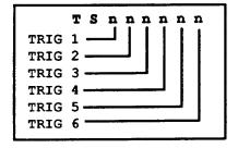
Since the TS command is immediate, the host controller can determine the status of the trigger inputs at any time, even during execution of other commands. You can use this command to make sure that your trigger pattern is met, when you have issued the Trigger (TR) command.
