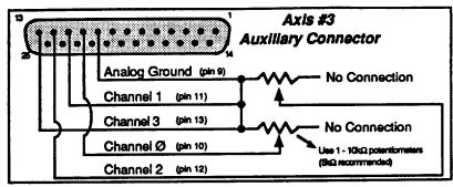
Axis 3 Aux. Connector: Typical Joystick Input Circuit
