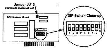
The DIP switches are negative true in that any switch in the position marked ON has a binary value of zero. Switches that are OFF have a non-zero binary value. The sum of the binary values of DIP switches 1 through 8 is the board's base address. The binary values assigned to each of the eight DIP switches are listed in the table below.
