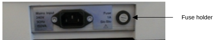
Figure 150 The position of the mains fuse
