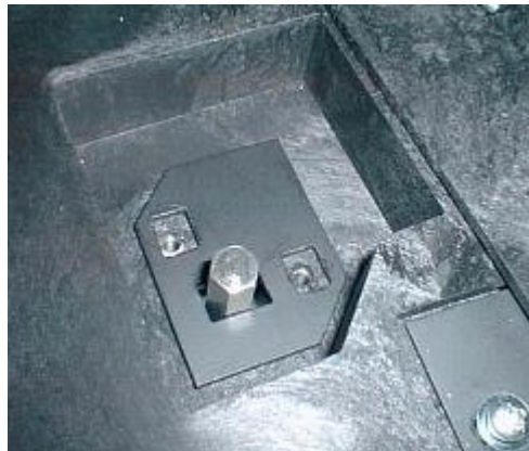
Figure 146 Replacing the shipping clamp plates
