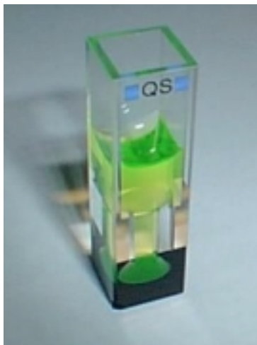
Figure 34 The stirred semi-micro cuvette
