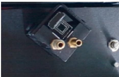
Figure 33 Inserting the semi-micro cuvette
