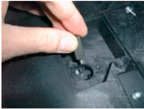
Figure 145 Inserting the shipping clamp screws
